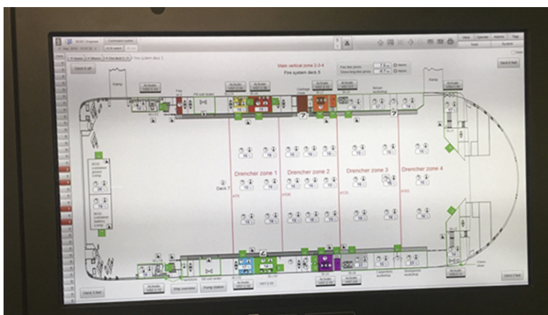
Figure 1: The Fire Resource Management Centre (FRMC) of the Stena Jutlandica Ro/Ro vessel will be augmented with A4IoT to enable real-time tracking of fire hazards and to guide trained personnel in controlling them.
